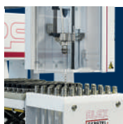
Automated Liner Exchange
