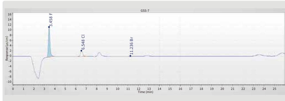
Detection of halogens and sulfate in coal mine
