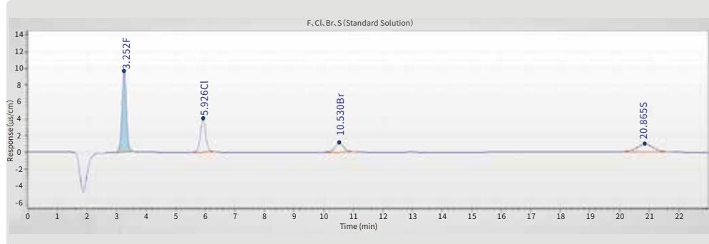
Detection of halogens and sulfur in textile
