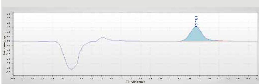
Detection of perchlorate in water (0.5mg/L)
