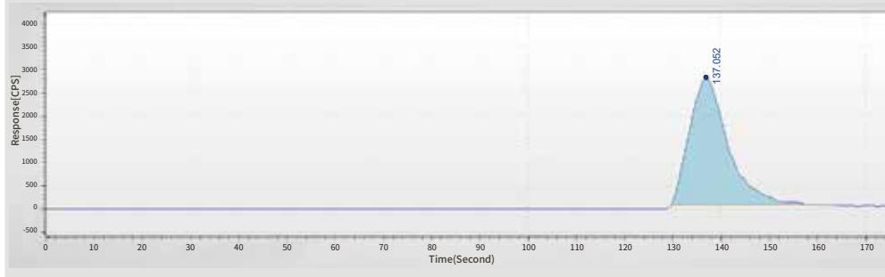
Detection of uranium in seawater by chelate chromatography-ICPMS( 3 $\mu$ g/L)
