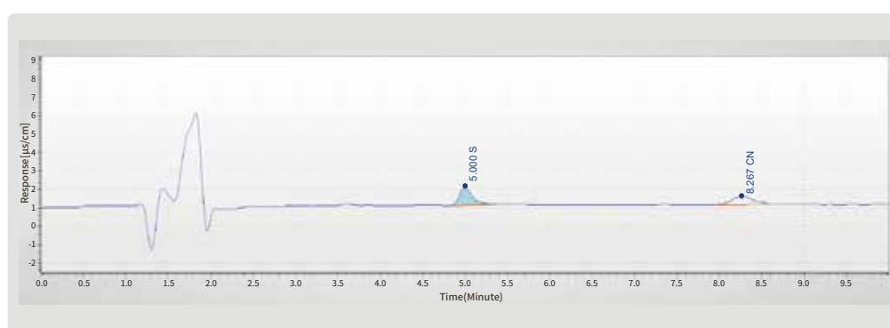
Detection of Sulfide and cyanide in waste water and solid waste (Direct current ampere detector, 1  $\mu\text{g/L}$ )
