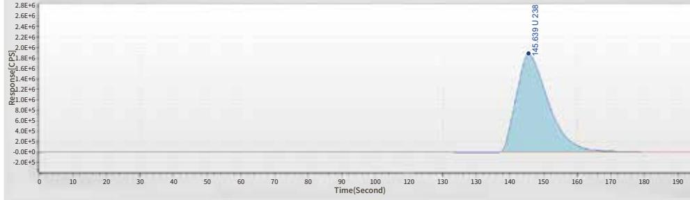
Detection of trivalent chromium and hexavalent chromium by LC-ICP-MS
