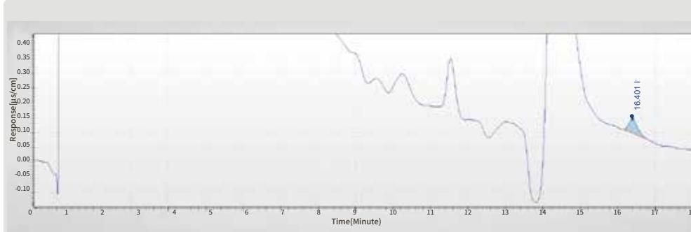
Nitrite salt derivatization method: Nitrite salts in seawater (post-column derivatization)
